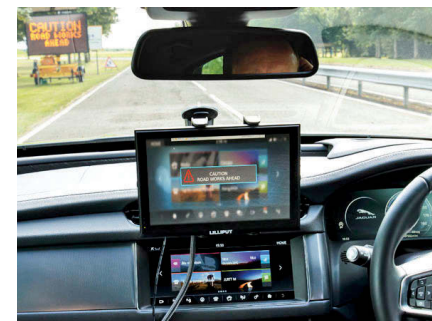
The over-horizon warning identifies hazards that are not yet in sight.
