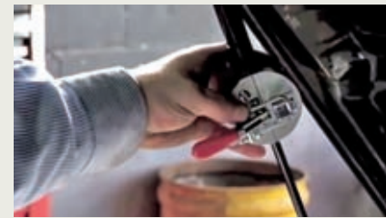
ShockLock clamps onto failing gas struts to keep the hood or trunk lid up.
