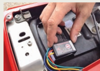
GearBrake's safety module flashes the brake lights whenever the vehicle slows.
