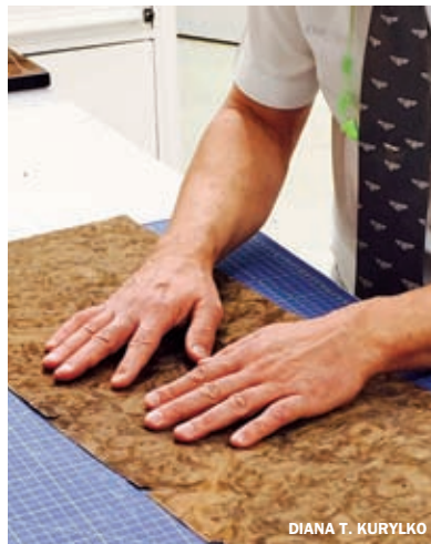
John Fisher, the Bentley plant's wood shop operations manager, matches paper-thin veneer for interiors.
