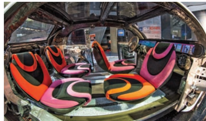
The concept car created by Clemson University students for General Motors features swivel seating for a denlike setting.
