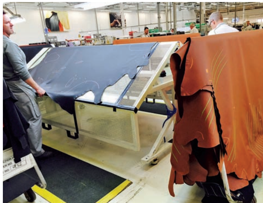
Workers at Bentley Motors' Pym Lane plant in Crewe, England, mark flaws in bull hides that will have to be cut out. Bentley won't use leather with imperfections.
