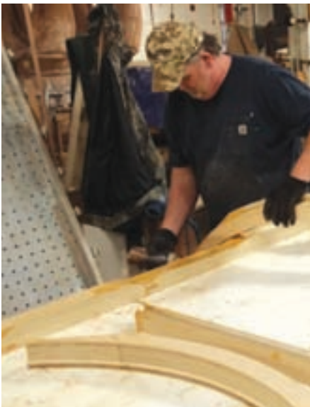
THE MINNESOTA STATE CAPITOL'S NEW WINDOWS NEEDED TO REPLICATE THE HISTORIC WINDOWS, BE ENERGY EFFICIENT AND OPERABLE. TO MATCH THE CAPITOL'S INTERIOR WOOD, 100-PLUS-YEAR-OLD LOGS WERE FOUND IN IDAHO LAKES, MILLED AND STAINED.
