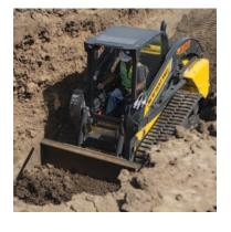
trols. These engines meet the Tier 4-Final emissions mandate with a maintenance-free DOC solution that eliminates the need for a diesel particulate filter (DPF).
