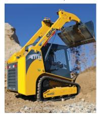
GEN:2. The RT Series offers the Ideal-Trax Automatic Track Tensioning System. This system eliminates manual track tensioning and increases the life of the tracks, sprockets and bearings due to the relief of track tension when the engine is shut off. This system saves the suggested 10-15 minute track tension checks that are recommended every 50 hours and the 30-45 minute tension readjustments required approximately every 300-400 hours depending on usage, Gehl says.
