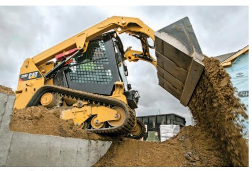
Keeping the undercarriage clean and free from premature wear is a key to keeping operating costs down.
