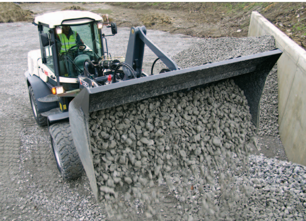
A Terex TL120 charges a pile of gravel. Manufacturers have been bringing hydrostatic drive to smaller loaders like this one.
