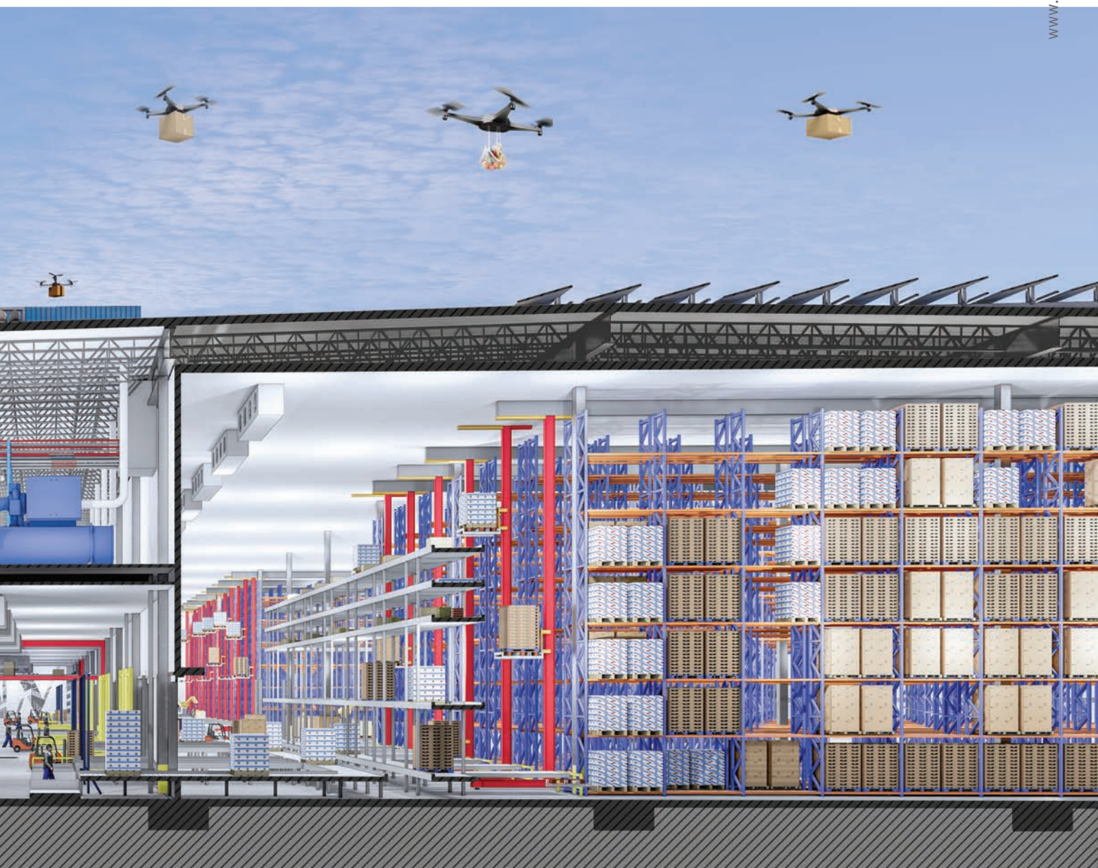
A section view of a cold-ready building showing refrigerated storage, the cold dock and the equipment mezzanine.
