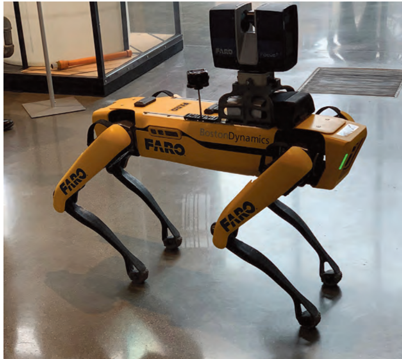
Boston Dynamics' Spot robot is 33 inches tall, weighs about 60 pounds and can move at a top speed of about 3.5 miles per hour.
