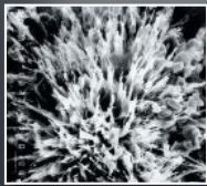
Xypex Crystallization (Mature)
