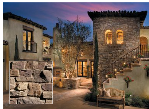
The extensive use of stone, specifically the rustic rubble blend combined with a heavy overgrout application, replicates the centuries old dwellings found in Europe. Photo courtesy of Eldorado Stone
