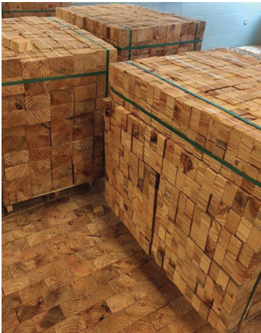
End-grain blocks should be mixed up (as shown on page 32) and acclimated before installation; these pine blocks are at a Connecticut school.
