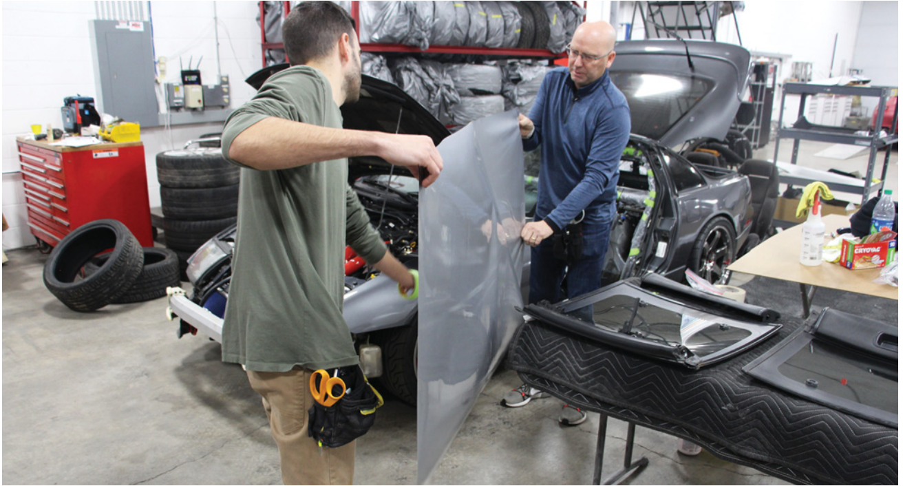
Sign Edge installer Dan Parker (left) and Hagen prepare to fit a satin gray vinyl wrap over the front of a vehicle.
