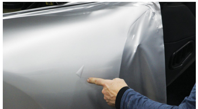
Hagen points out an air bubble that can form during an install.
