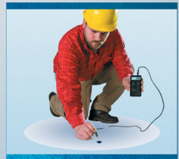
Concrete in-situ RH Test
