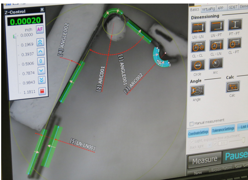
Figure 5 A stamped component is measured to be within tolerance. The green and light-blue marks show the key areas for measurement.
