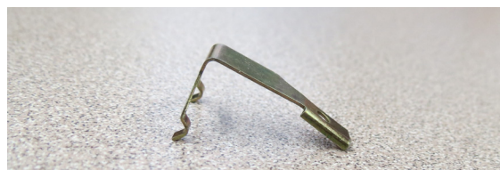
Figure 2 This stamped component doesn't lie flat, so it needs a custom fixture to be measured. That's where 3-D printing comes into play.
