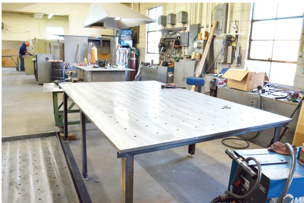
Figure 5 Stephen Hedlund had a custom welding table made so that fabricators can construct fixtures quickly and change over to the next job in a few minutes.
