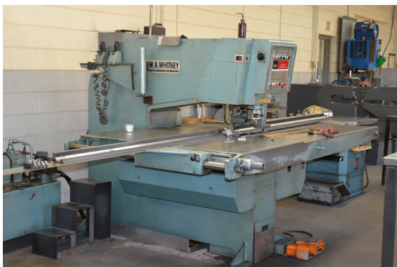
Figure 4 Punching out blanks on Co-Lin's older punch presses, on which the operator has to hand-crank the punch into position and then engage the punch with a foot pedal, simply can't compete with having them laser-cut by another company.
