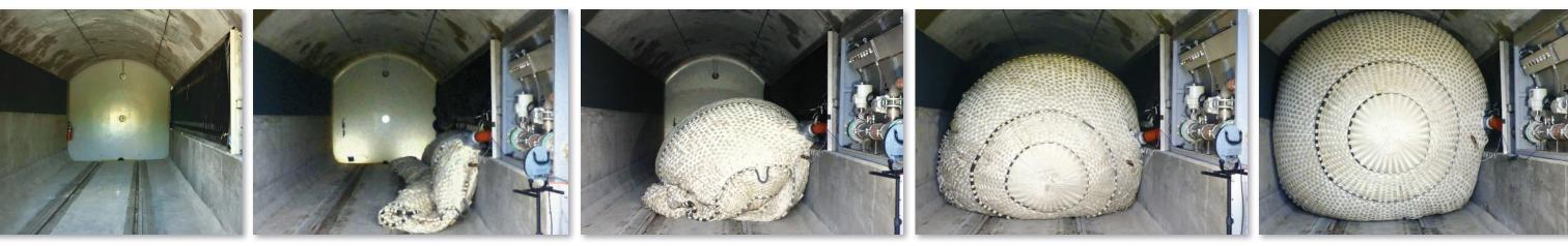
neered fabric systems based in Frederica, Delaware; the U.S. Department of Energy's Pacific Northwest National Laboratory, in Richland, Washington; and West Virginia University. Their decade-long effort to develop a plug that would be capable of stopping floodwaters from entering subway tunnels and could be stored at
