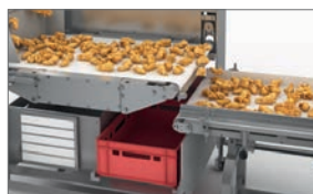
Contaminated products will be ejected into bin by reversing outfeed belt
