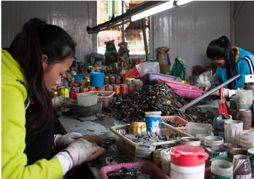
Hand sorting. Fewer than a dozen trained workers can sort through some 2 tonnes to 3 tonnes of coins each day, quickly dividing global coins by country and denomination.
