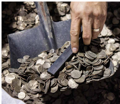
Unsealed. Wealthy Max Ltd. publicly opened and sampled 13 tonnes of mutilated U.S. coins in Hong Kong. The pennies, dimes, quarters and half dollars come from piles of metal generated by automotive shredders and via incinerated waste streams.
