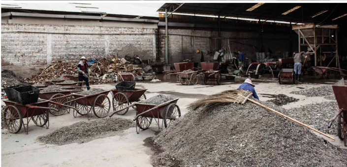
▲ Reclamation chain. Shipments of zorba and other mixed metal waste pass through a series of screening and flotation techniques before being hand sorted by metal grade. Coins go to coin recyclers, while the other metals will be grouped and either traded or melted and cast into ingots.
