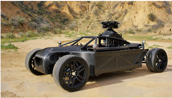
The adjustable Blackbird can change digital skin and pose as practically any car for commercials.
