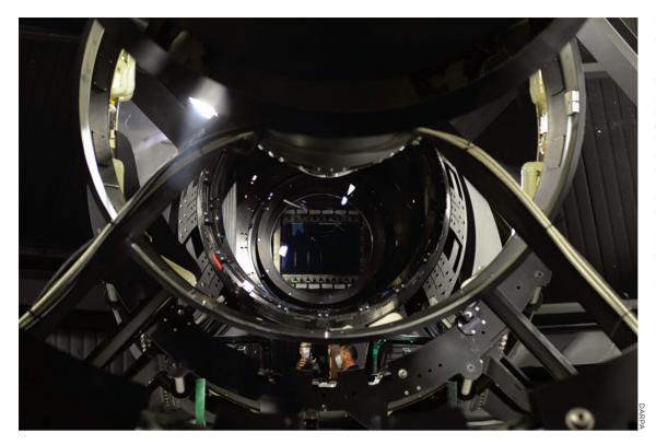
The DARPAdesigned Space Surveillance Telescope will test enhanced small-objectdetection algorithms for objects in geosynchronous orbit. At center is its wide field camera. In 2013, the U.S. and Australia agreed to relocate the telescope from New Mexico to western Australia, but the move has not been made yet.
