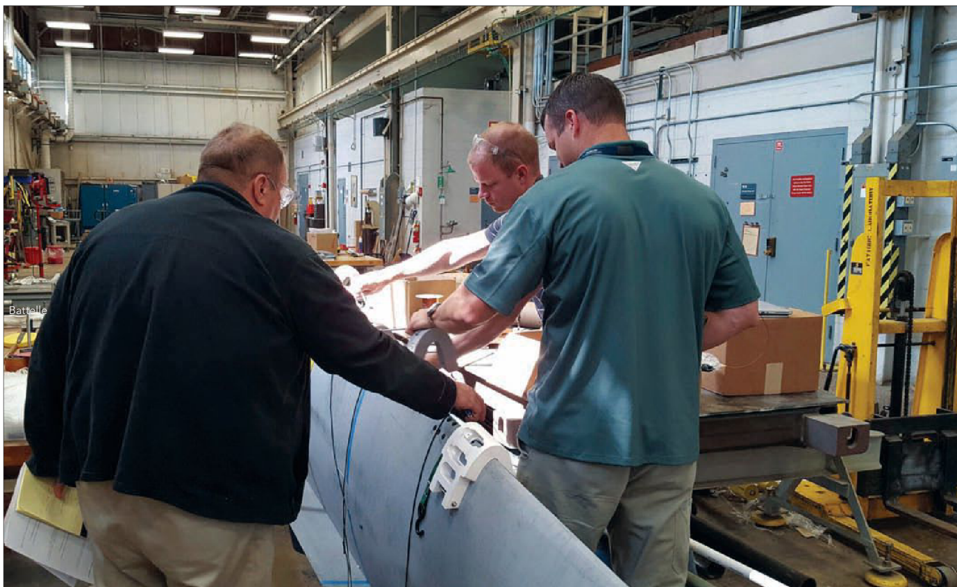
Battelle employees attach an alignment drill jig to a wing section in an engineering lab in Columbus, Ohio. Holes were drilled to run wires to carry current to melt ice.
